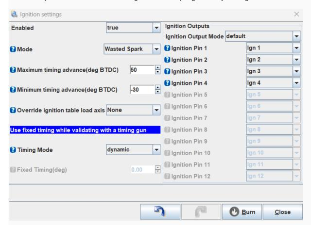
A pair of protection settings are in place, Maximum advance or minimum advance, this is to delimit how high the advance can be under all scenarios, or how negative it can be.
