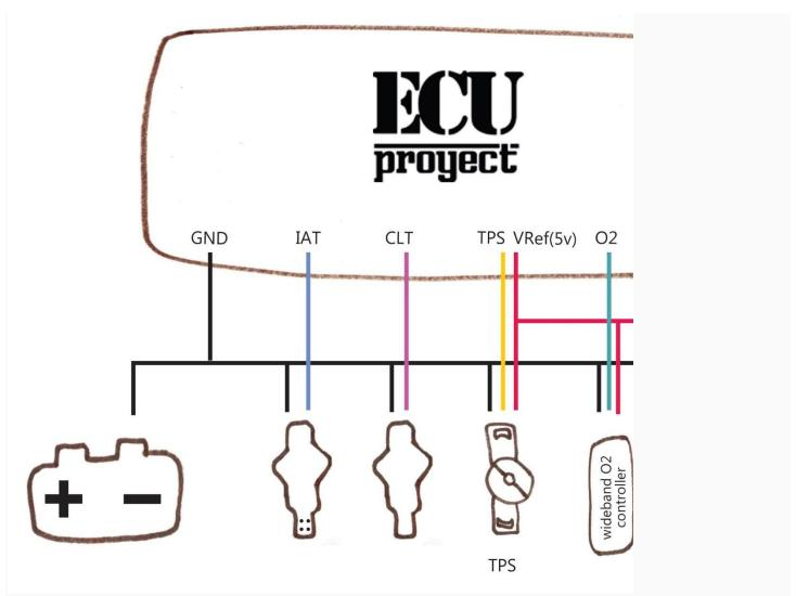
Notes: Use of 2-wire temperature sensors is recommended. While 1-wire sensors will work, they are almost always considerably less accurate.
