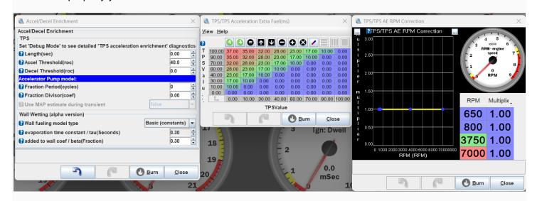
The enrichment curve included with the ProyectECU base tune is a good starting point for most engines, but some adjustments are normal depending on injector size, throttle diameter, etc.
