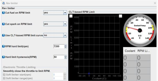
We can select if we want RPM limiter by spark cut and/or fuel cut. The recommendation is of course spark cut, this creates a nice explosive rpm limiter.
