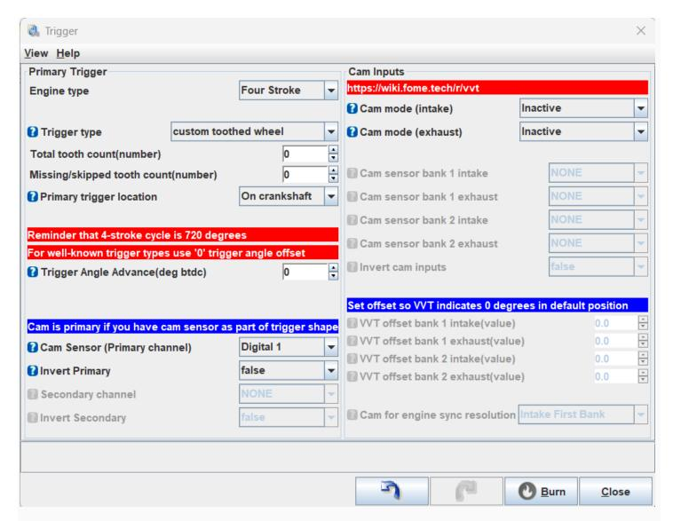
Theres a selection for engine type: Four or two stroke. And the trigger type, here the selection of triggers varies from a basic distributor to some complex like a VQ35.
